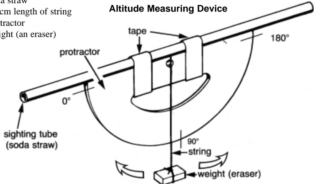
The device should look like the one in the diagram. Tape the straw across the top of the protractor as shown. The straw will act as a sighting tube. Secure the string to the protractor, slipping it under the straw and taping it to the back of the protractor. Tie the eraser at the opposite end of the string, so that it can act as a weight.
