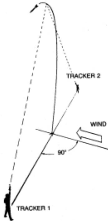
The two results are averaged, and the average is used as the height reached. Usually both heights will be thrown out if they are not within ten percent of each other. This assumes that at least one of the tracking stations made a mistake and the results cannot be considered reliable.
