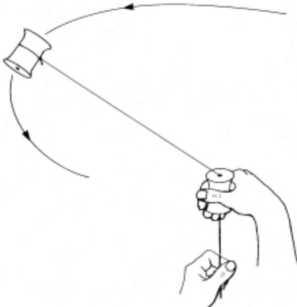
Moving objects possess momentum. The amount of momentum an object has is determined by multiplying its mass times its velocity. For example, a 100 pound satellite moving at 4.85 miles per second, which is the orbital velocity for a satellite in circular orbit at a height of 100 miles above the Earth's surface, will have a momentum of 2,560,800 foot-pounds/second. (100 lbs. x 4.85 miles/second x 5280 feet/mile=2,560,800 ft.lbs./second).
