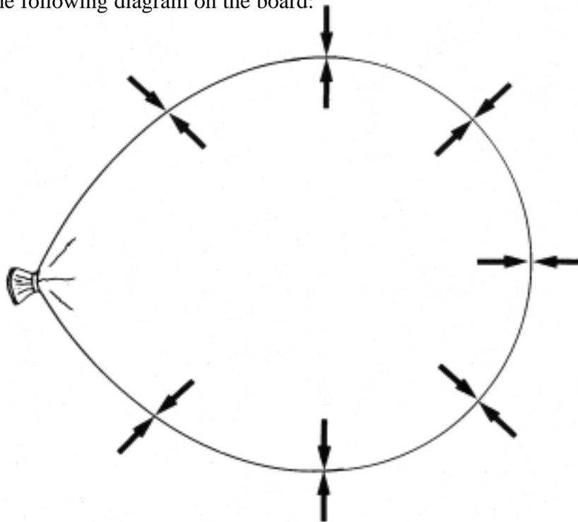
This diagram shows that air inside the balloon is compressed by the balloon's rubber walls. The air pushes back so that the inward and outward pressing forces are balanced.
