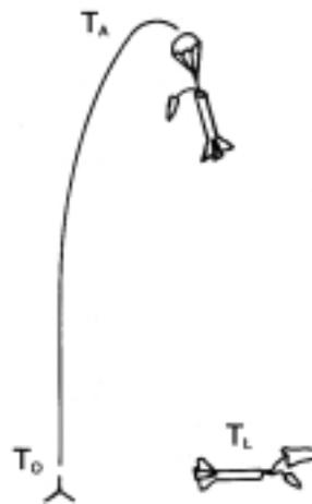
On the diagram, distance traveled is the distance between  $T_O$  and  $T_A$  (launch to apogee). That is the altitude or height the rocket reached at apogee.
