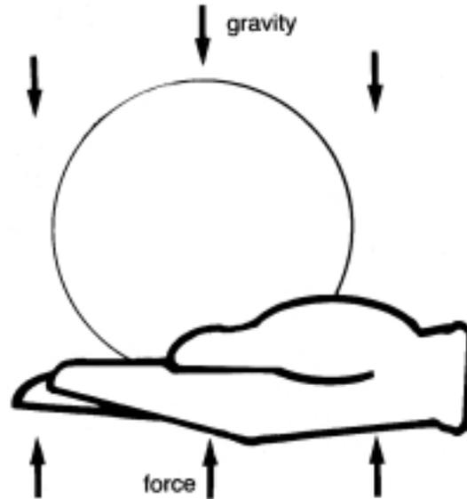
The ball changes from a state of rest, being acted upon by balanced forces to a state of motion, being acted upon by unbalanced forces when you let the ball go or you move your hand upward. When an object is at rest, it takes an unbalanced force to make it move.
