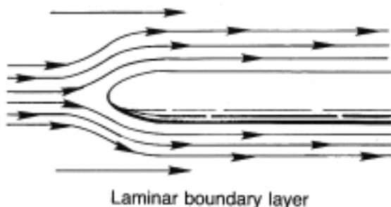
Drag increases as velocity or speed increases. The drag experienced by the object directly varies with the square of the velocity of the moving object. The basic drag formula for the effect of velocity on drag is:
