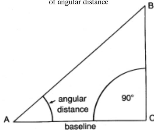
If we assume that the rocket flight is vertical, we can call angle C a right angle, 90 degrees. B is equal to 90 degrees minus A, because the sum of the angles in a triangle is 180 degrees. To find the distance from C to B or the height the rocket
