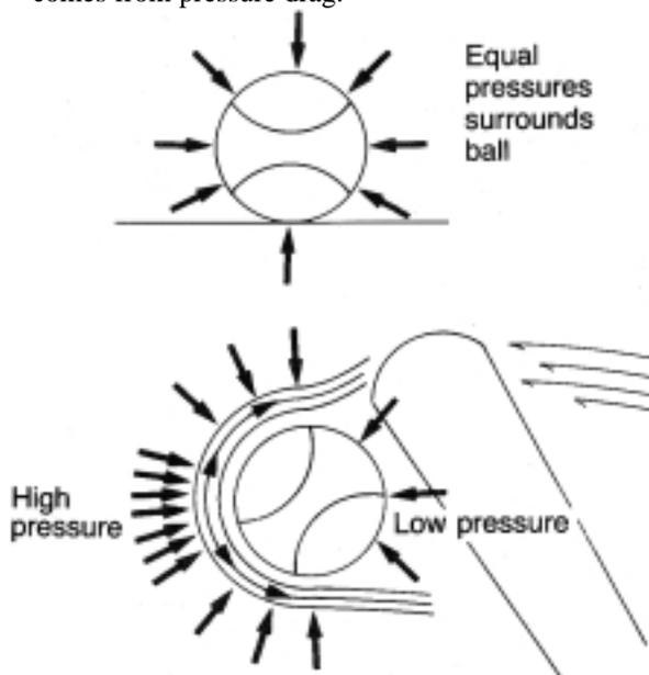
Pressure drag is the retarding force caused by the imbalance of air pressures on a moving object. Pressures on a moving object vary with the object's speed, direction of motion and its size and shape.
