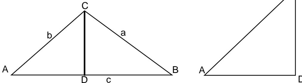
The altitude of the rocket is the distance from D to C in the diagram. The angle formed by the meeting of AB and CD is a right angle. The sine of an angle in a right triangle is the relation of the opposite side to the hypotenuse. We want to determine the value of the opposite, CD.
