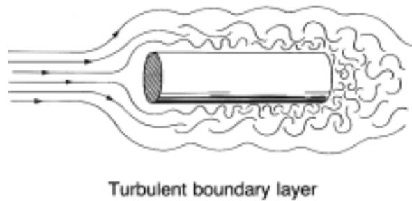
To prevent flows from separating, it is essential to use aerodynamic shapes that are rounded gently and never have any sharp changes in direction. When there are sharp changes, the viscosity of the air makes the flow resist these changes in directions and forces the flow to break away.
