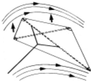
Lift is generated by *relative wind*. Relative wind is the motion in the air in relation to an object, such as a kite in a breeze. It can also be created by running with a kite, if no wind is blowing.
