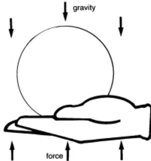
The ball changes from a state of rest, being acted upon by balanced forces to a state of motion, being acted upon by unbalanced forces when you let the ball go or when you move your hand upward. When an object is at rest, it takes an unbalanced force to make it move.
