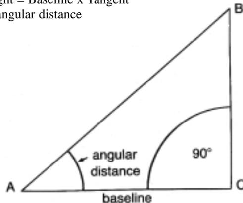
If we assume that the rocket flight is vertical, we can call angle C a right angle, 90°. B is equal to 90° minus A because the sum of the angles in a triangle is 180°. To find the distance from C to B or the height the rocket reached, take the tangent of Angle A times the distance along the baseline, side AC.
