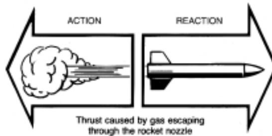
The sides of the combustion chamber prevent the gases from escaping sideways. The gases cannot escape forward. The only opening to the outside is the nozzle. A tremendous volume of hot gases is produced as the fuel is burned. These hot gases have mass and this mass can escape only through the rocket's nozzle at high velocity. The gases have a large momentum.
