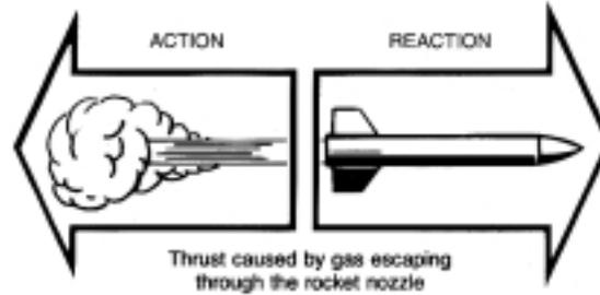
The escaping gases acquire momentum due to the action. The reaction gives momentum to the rocket which is equal but opposite in direction. The large mass of the rocket is given a small velocity so that the momentum (reaction) of the rocket is equal to the momentum (action) of the escaping low-mass, high-velocity gases.
