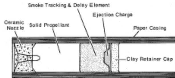
Model rocket engines are manufactured in a range of sizes. They come in over 30 varieties, each one varying in total impulse, average thrust, thrusting time and time of delay between propellant burnout and activation of the ejection charge.
