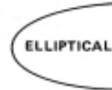
Advantages: most aerodynamically efficient shape available and hence it has the lowest drag
