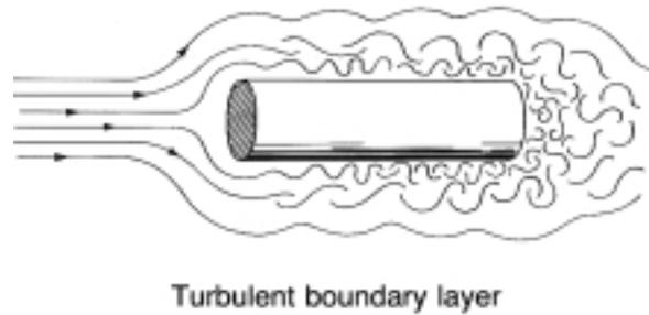
Drag increases as velocity or speed increases. The drag experienced by the object directly varies with the square of the velocity of the moving object.
