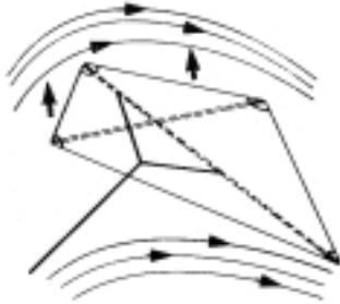
Lift is generated by *relative wind*. Relative wind is the motion in air in relation to an object, such as a kite in a breeze. It can also be created by running with a kite, if no wind is blowing.
