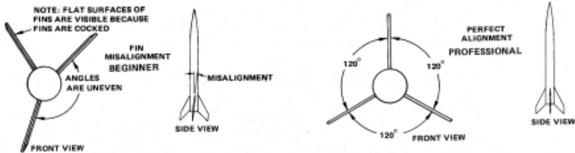
A. Describe the effects of rough cut leading edges, trailing edges and unsanded and unpainted surfaces on the performance of a model rocket in relation to aerodynamic forces.
