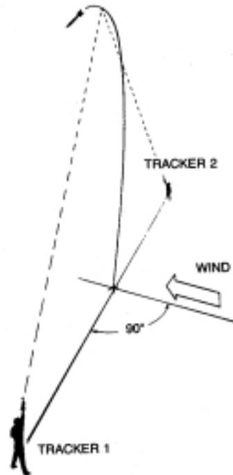
Each tracking station takes its own measurements of the angle reached. Both heights are calculated. The two results are averaged, and the average is used at the height reached. Usually both heights will be thrown out if they are not within ten percent of each other. This assumes that at least one of the tracking stations made a mistake and the results cannot be considered reliable.
