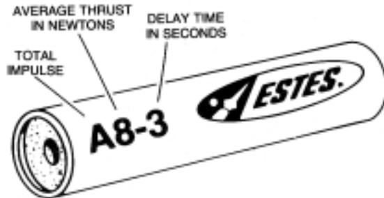
The engine code on each engine consists of a letter, a number and another number preceded by a dash. The letter indicates the total impulse or power of the engine. The number indicates the average thrust of the engine. This value is in newtons. The last number is the delay time in seconds between the time of the engine's burnout and the activation of the ejection charge
