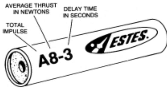
The engine code on each engine consists of a letter, a number and another number preceded by a dash. The letter indicates the average thrust of the engine. This value is in newtons. The last number is the delay time in seconds between the time of the engine's burnout and the activation of the ejection charge.
