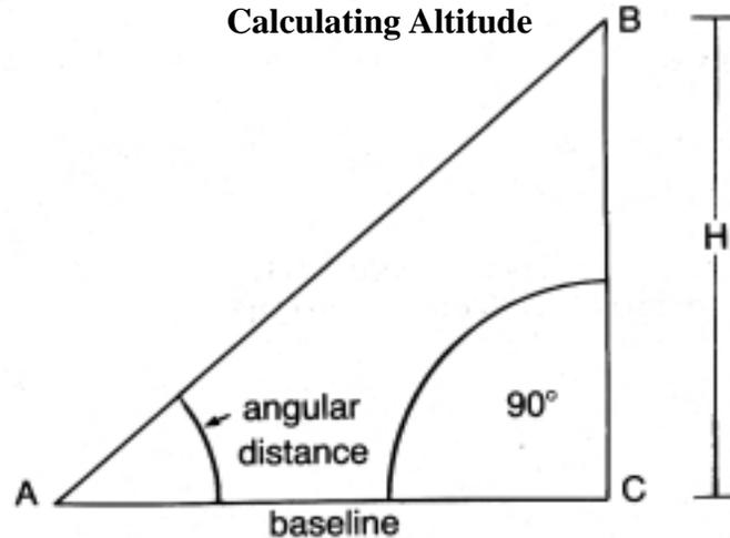
The rocket is being launched at C. You are standing at A with your altitude tracking device. You are trying to determine the angle at A by tracking your rocket as it travels from C to B. B is apogee and that is where you need to note where the string is on the protractor. **Remember, if you are using a homemade tracker you have to subtract that number from 90° in order to get the angular distance. If you are using an Estes AltiTrak™ you can read the angular distance directly off the AltiTrak™.**
