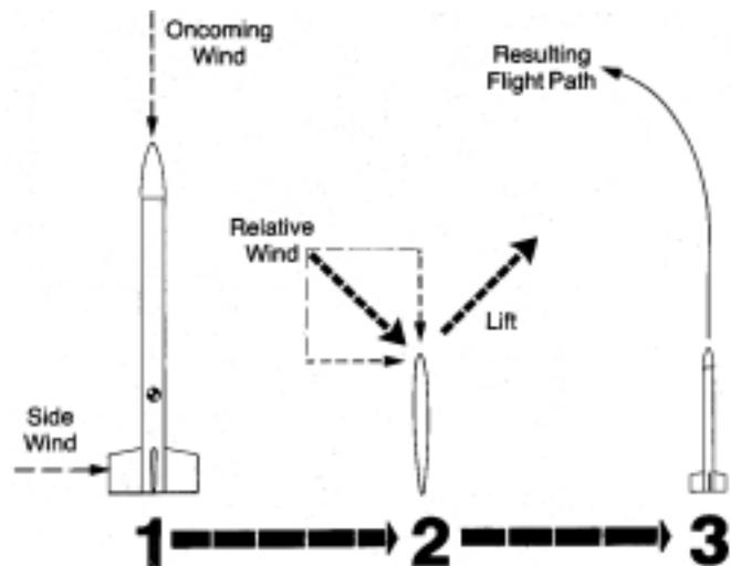
As you can see, the fin is the stabilizing and guiding unit of a model rocket. It should be in a symmetrical form of three, four or possibly more fins and made of reinforced paper, balsa or plastic. The fin is an aerodynamic surface projecting from the rocket body.
