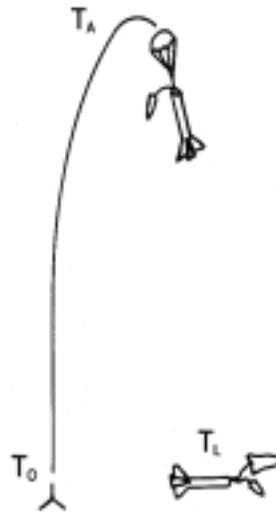
On the diagram, distance traveled is the distance between  $T_O$  and  $T_A$  (launch to apogee). That is the altitude or height the rocket reached at apogee.
