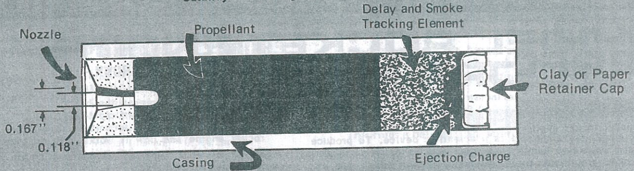
Cutaway of C6-5 engine.
