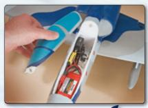
Magnet-secured hatch covers provide easy access to the battery. There's room to install a wide range of battery sizes.
