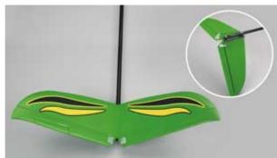
The V-tail design makes use of pushrods and control surfaces for precise flight control!
