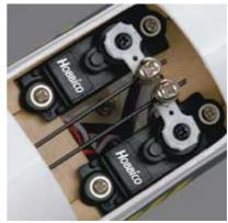
The lightweight, micro-sized servos that come with the Aero Voyager provide precise flight control.
