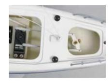
3. An installed steering servo provides control of the Paradise's rudder. The rudder control arm is located in its own hull compartment, which features a quick-access hatch topped off by a replica steering wheel.
