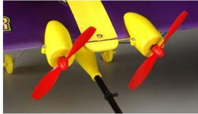
The Sky Screamer's twin motors and props are used for both thrust and steering, and are preinstalled for convenience. The rear-facing, "pusher" design helps protect the props from damage.
