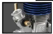
The dual-needle carbs on all .18 CV-R engines are screwdriver-adjustable, and the fuel inlet rotates a full 360 degrees for mounting options and fueling convenience.
