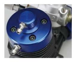
With the intake mounted directly on the plug, cooling water is channeled to the center of the head — the engine's hottest point — before exiting.
