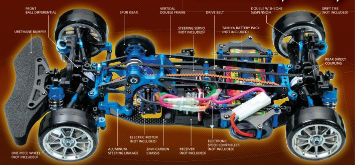
The TA05-VDF is specially designed for top-level drift performance. Its unique chassis layout, including the carbon fiber Vertical Double Frame, provides optimum weight distribution and balance. A proven belt-driven 4WD system efficiently transmits the motor power while the 4-wheel double wishbone suspension equipped with short reversible suspension arms and TRF dampers gives the chassis superior control.
