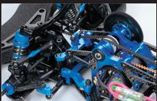
Suspension area features TA05 bulkheads, short reversible suspension arms, and TRF416 uprights. Proven 2-belt driven drivetrain features new drive belts and a belt tensioner.
