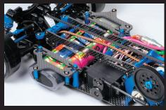
Adjustable battery holders enable attachment of Tamiya Ni-Cd, Ni-MH, and LF battery packs (battery packs can also be secured with glass tape). R/C units are placed centrally to achieve improved weight distribution.
